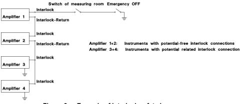
Figure 3: Example of interlock safety loops
