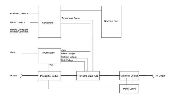
Figure 1: Amplifier block diagram
