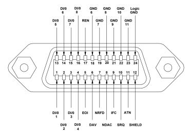
Figure 7: Pin assignment of IEEE connector
